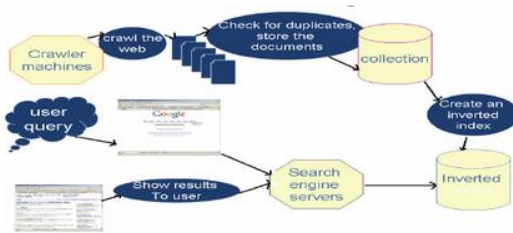
Figure 3. Standard Web Search Engine Architecture
